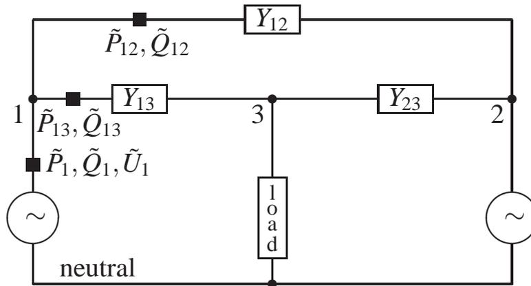
Fig. 9.2. Three-bus power system state estimation problem.
