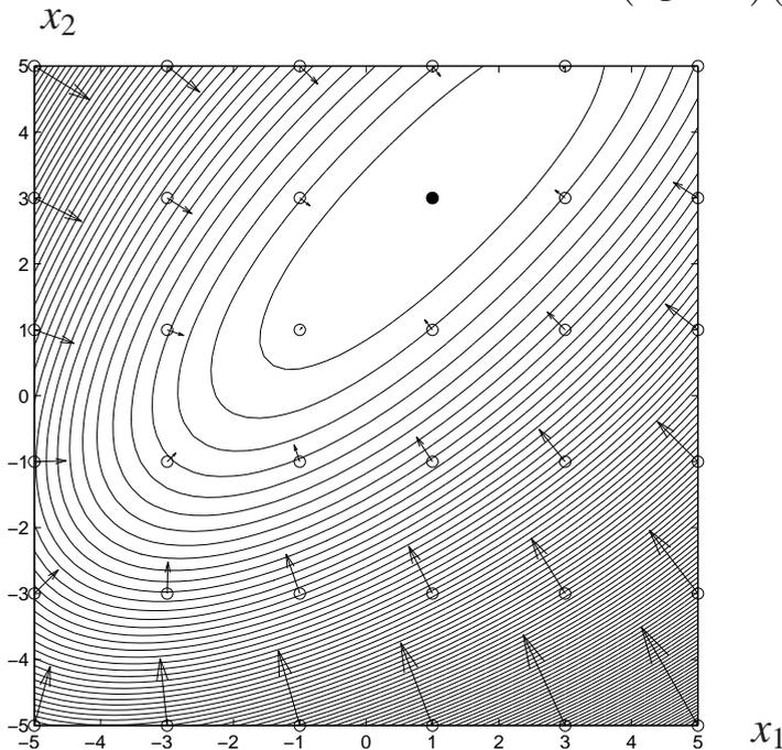
Fig. 10.11. Scaled versions of the steepest descent step directions for an objective, defined in (10.9), with contour sets that are perturbed eccentric ellipses. The contours of the function decrease towards  $x^* = \begin{bmatrix} 1 \\ 3 \end{bmatrix}$ , which is shown as a ●.
