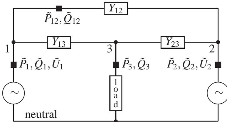
Fig. 11.3. The three-bus power system state estimation problem with spread out measurements repeated from Figure 9.3.
