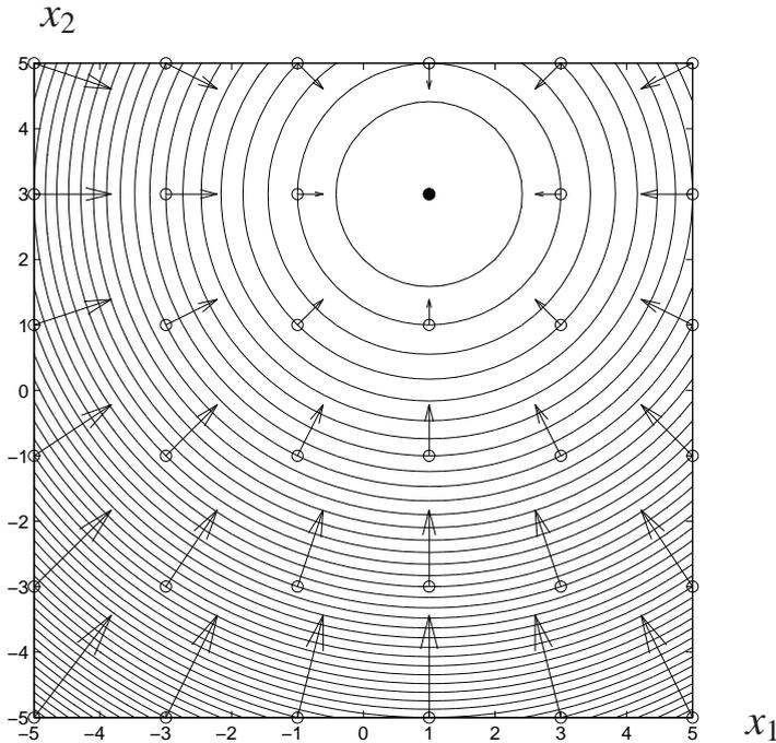
Fig. 10.2. Steepest descent directions for a function at various points. The contours of the function decrease towards  $x^* = \begin{bmatrix} 1 \\ 3 \end{bmatrix}$ , which is shown as a  $\bullet$ .
