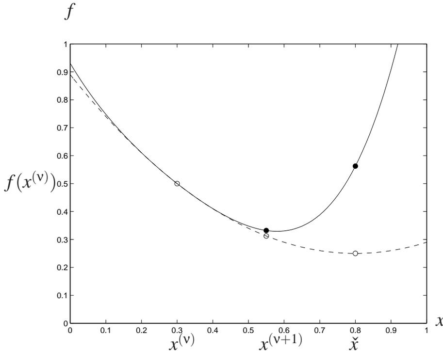
Fig. 10.17. The need for a step-size rule. The function  $f$  is illustrated with a solid line together with a quadratic approximation to it, illustrated as a dashed line. The quadratic approximation is a second-order Taylor approximation of  $f$  about  $x^{(v)} = 0.3$ .
