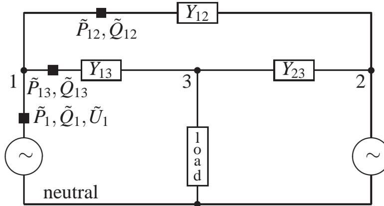
Fig. 11.2. The three-bus power system state estimation problem, repeated from Figure 9.2.
