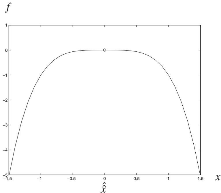
Fig. 10.7. A critical point  $\hat{\hat{x}} = 0$ , illustrated by the  $\circ$ , where the second derivative matrix is positive semi-definite at  $\hat{\hat{x}}$  yet the point is not a minimizer.
