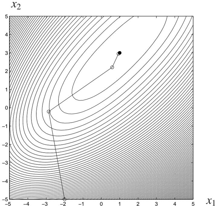
Fig. 10.16. Progress of iterations, shown as  $\circ$ , using Newton–Raphson step directions for an objective, defined in (10.9), with contour sets that are perturbed eccentric ellipses. The contours of the function decrease towards  $x^* = \begin{bmatrix} 1 \\ 3 \end{bmatrix}$ , which is shown as a  $\bullet$ . The initial guess was  $x^{(0)} = \begin{bmatrix} -2 \\ -5 \end{bmatrix}$ .
