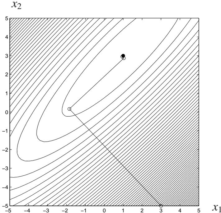
Fig. 10.9. Progress of iterations, shown as  $\circ$ , using steepest descent step directions for an objective, defined in (10.8), with contour sets that are highly eccentric ellipses. The contours of the function decrease towards  $x^* = \begin{bmatrix} 1 \\ 3 \end{bmatrix}$ , which is shown as a  $\bullet$ . The initial guess was  $x^{(0)} = \begin{bmatrix} 3 \\ -5 \end{bmatrix}$ .
