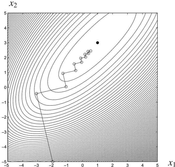
Fig. 10.13. Progress of iterations, shown as  $\circ$ , using steepest descent step directions for an objective, defined in (10.9), with contour sets that are perturbed eccentric ellipses. The contours of the function decrease towards  $x^* = \begin{bmatrix} 1 \\ 3 \end{bmatrix}$ , which is shown as a  $\bullet$ . The initial guess was  $x^{(0)} = \begin{bmatrix} -2 \\ -5 \end{bmatrix}$ .
