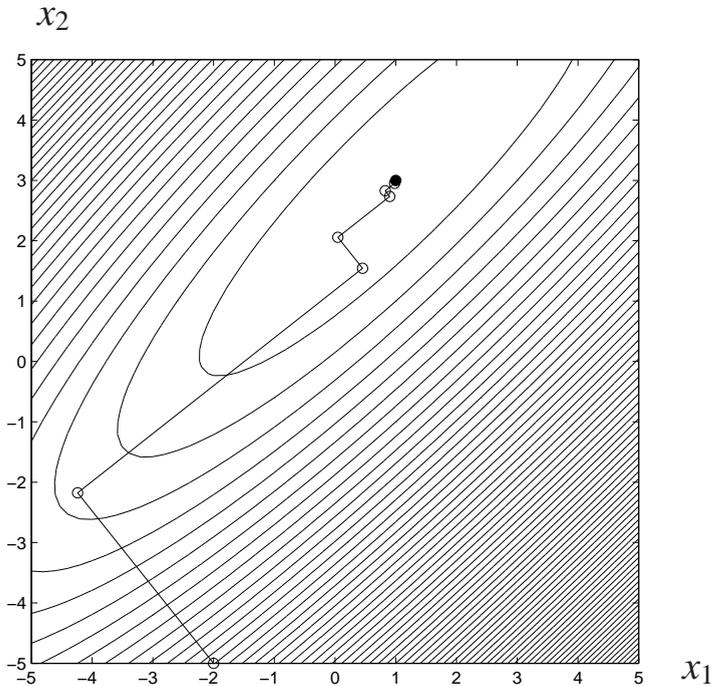
Fig. 10.10. Progress of iterations, shown as  $\circ$ , using steepest descent step directions for an objective, defined in (10.8), with contour sets that are highly eccentric ellipses. The contours of the function decrease towards  $x^* = \begin{bmatrix} 1 \\ 3 \end{bmatrix}$ , which is shown as a  $\bullet$ . The initial guess was  $x^{(0)} = \begin{bmatrix} -2 \\ -5 \end{bmatrix}$ .
