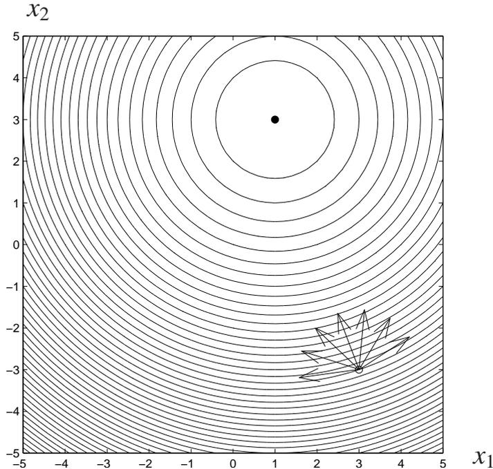
Fig. 10.3. Various descent directions for a function at a particular point  $\hat{x} = \begin{bmatrix} 3 \\ -3 \end{bmatrix}$ . The contours decrease towards the point  $x^* = \begin{bmatrix} 1 \\ 3 \end{bmatrix}$ , which is shown as a  $\bullet$ .
