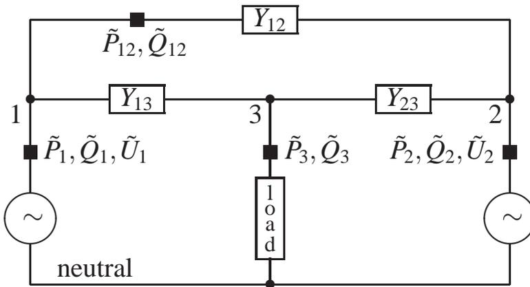
Fig. 9.3. Three-bus power system state estimation problem with spread out measurements.
