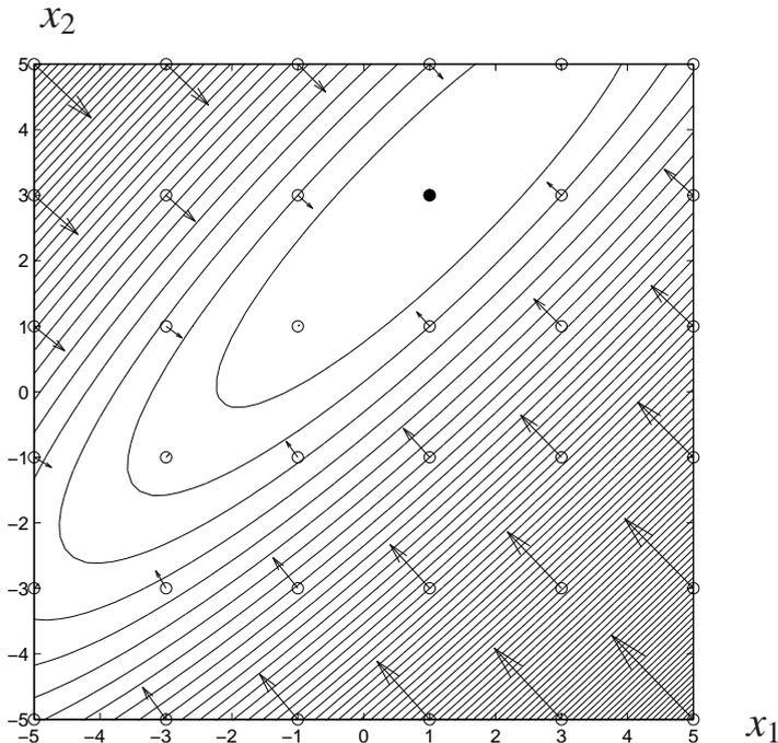
Fig. 10.8. Scaled versions of the steepest descent step directions for an objective, defined in (10.8), with contour sets that are highly eccentric ellipses. The contours of the function decrease towards  $x^* = \begin{bmatrix} 1 \\ 3 \end{bmatrix}$ , which is shown as a  $\bullet$ .
