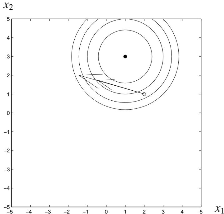
Fig. 10.1. Descent direction (shown as the longer arrow) for a function at a point  $\hat{x} = \begin{bmatrix} 2 \\ 1 \end{bmatrix}$ , shown as a  $\circ$ . The contours of the function decrease towards  $x^* = \begin{bmatrix} 1 \\ 3 \end{bmatrix}$ , which is shown as a  $\bullet$ .
