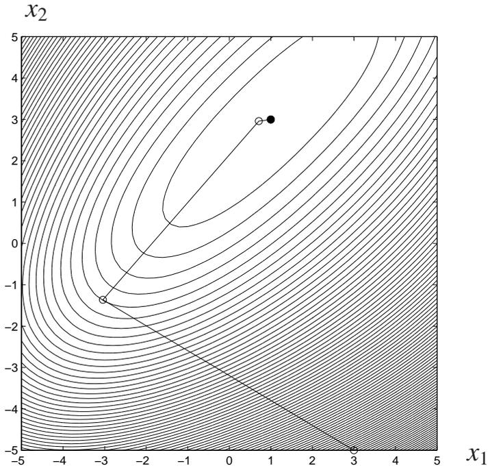
Fig. 10.15. Progress of iterations, shown as  $\circ$ , using Newton–Raphson step directions for an objective, defined in (10.9), with contour sets that are perturbed eccentric ellipses. The contours of the function decrease towards  $x^* = \begin{bmatrix} 1 \\ 3 \end{bmatrix}$ , which is shown as a  $\bullet$ . The initial guess was  $x^{(0)} = \begin{bmatrix} 3 \\ -5 \end{bmatrix}$ .
