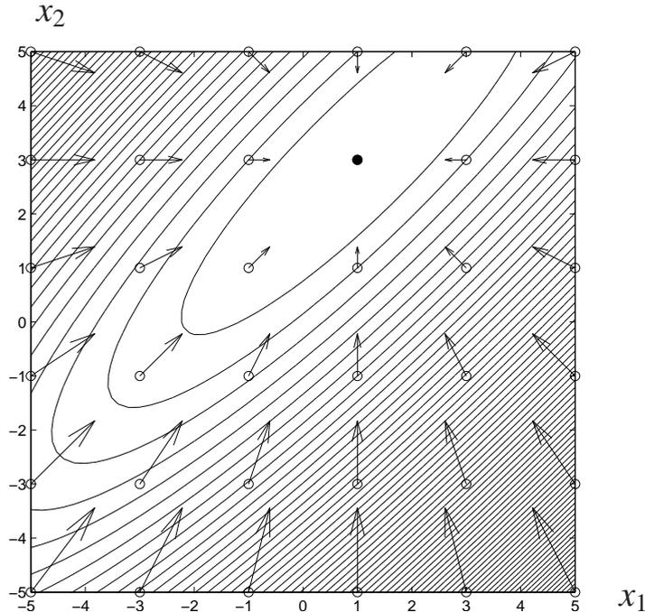
Fig. 10.14. Scaled versions of the Newton–Raphson step directions for an objective, defined in (10.8), with contour sets that are highly eccentric ellipses. The contours of the function decrease towards  $x^* = \begin{bmatrix} 1 \\ 3 \end{bmatrix}$ , which is shown as a  $\bullet$ .
