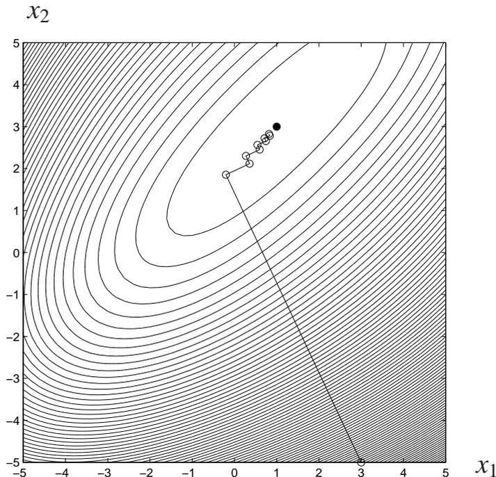
Fig. 10.12. Progress of iterations, shown as  $\circ$ , using steepest descent step directions for an objective, defined in (10.9), with contour sets that are perturbed eccentric ellipses. The contours of the function decrease towards  $x^* = \begin{bmatrix} 1 \\ 3 \end{bmatrix}$ , which is shown as a  $\bullet$ . The initial guess was  $x^{(0)} = \begin{bmatrix} 3 \\ -5 \end{bmatrix}$ .
