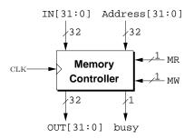
The busses are connected to the memory controller as follows.
